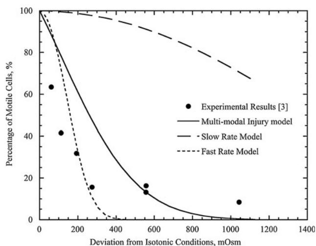
FIG. 7. Loss of motility during forced convective desiccation. Using motility results,<sup>3</sup> the models are used to predict loss of motility for forced convection desiccation. The model prediction is calculated from Eq. (1) and (4) for the first-order rate and multi-modal injury models, respectively.
